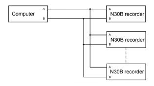
Fig. 15. Connection Way of the RS-485 Interface.
