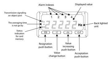
Fig. 5. Description of the recorder frontal plate.
